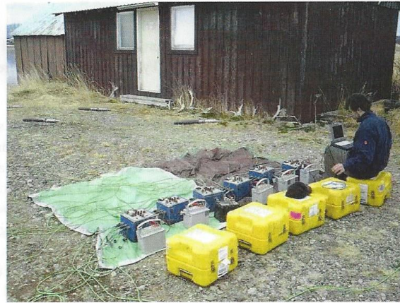
Exhibit 1. MT Survey Equipment (Acquisition and processing units and coils).
